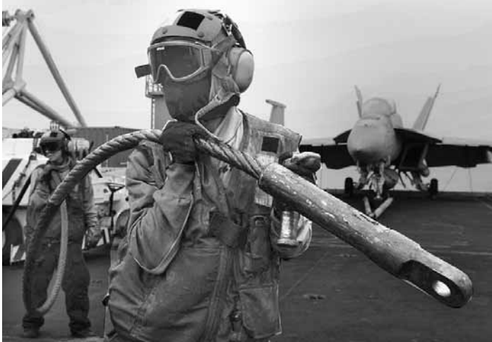
Aviation Boatswain's Mate (Equipment) Airman Megan E. Walker, left, and Aviation Boatswain's Mate Airman Kapri D. Ragin move a length of arresting gear wire on the flight deck of the aircraft carrier USS George H.W. Bush (CVN 77). (U.S. Navy photo by Mass Communication Specialist Seaman Apprentice Brian Read Castillo/Released)
